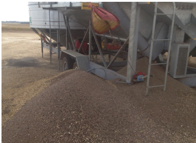
▲ Photo 1. A pile of small conical snails removed from canola using a 4-barrel rotary grain cleaner with 2.5mm slotted screens.
