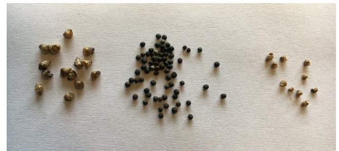
▲ Photo 2. Snails on the left were removed from the canola (centre) using a rotary grain cleaner with 2.5mm slotted screens. The snails on the right could not be removed using the same screens.
