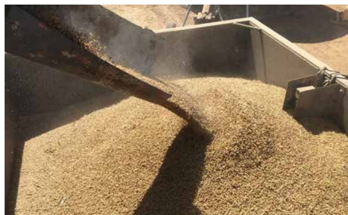
FIGURE 1. Barley moving from the auger into the hopper of the snail roller. A sensor ensures the hopper remains full to maximise grain turnover and improve snail removal.
