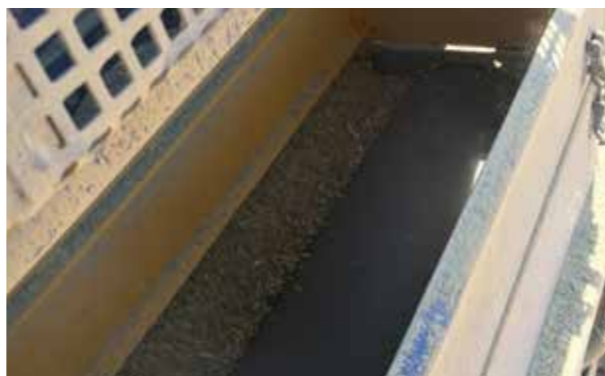
FIGURE 2. The barley flowing between the rollers during sampling. The roller temperature may need to be monitored to make sure it does not exceed 65°C. Using a gap of 0.8mm the roller temperature remained between 48-50°C.
