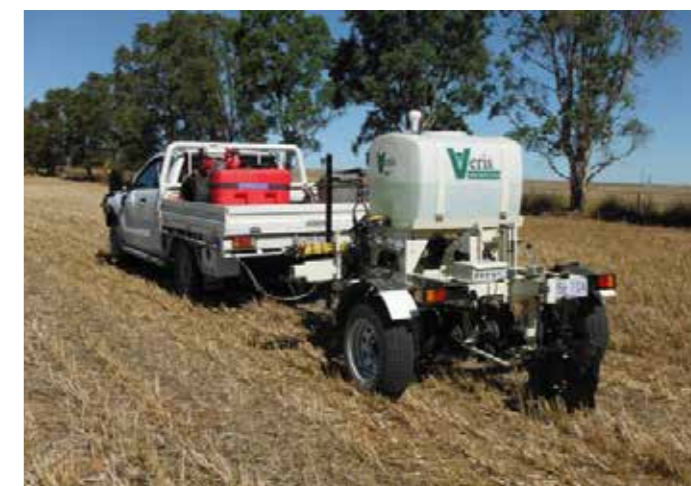
FIGURE 1. Veris On-the-go soil pH sensor (Source: Stock Journal, 2018)
