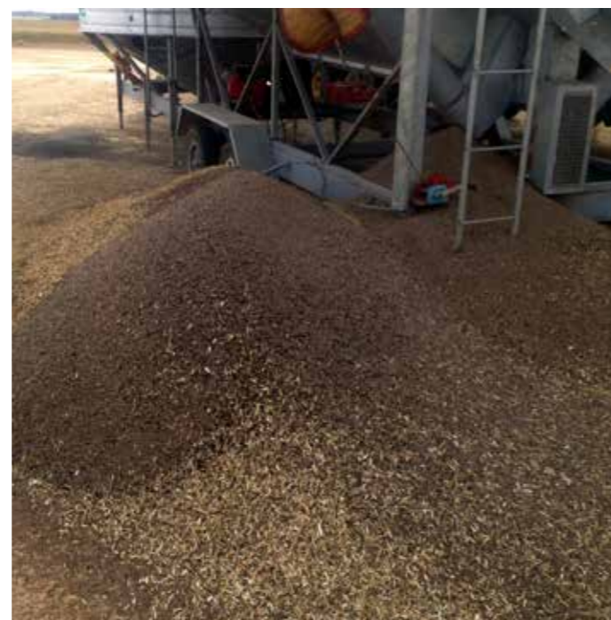
PHOTO 1. A pile of small conical snails removed from canola using a 4-barrel rotary grain cleaner with 2.5mm slotted screens.
