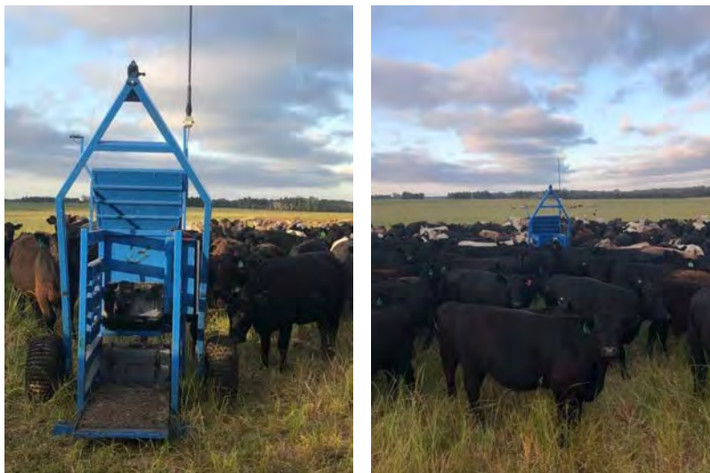
Figure 1. Optiweigh system on site at Kent Rochester's.
