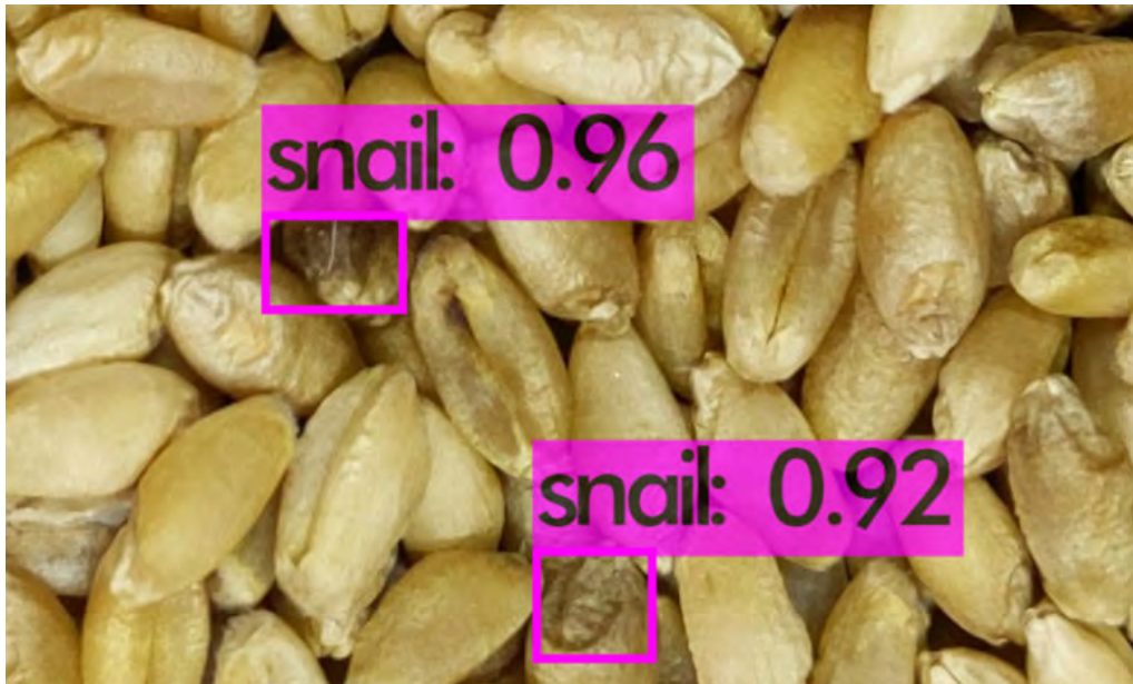
Figure 4: Grain defects that were misclassified as snails.
