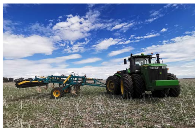
Figure 2: Image of Nufab deep ripper used to achieve an approximate 500mm deep amelioration.
