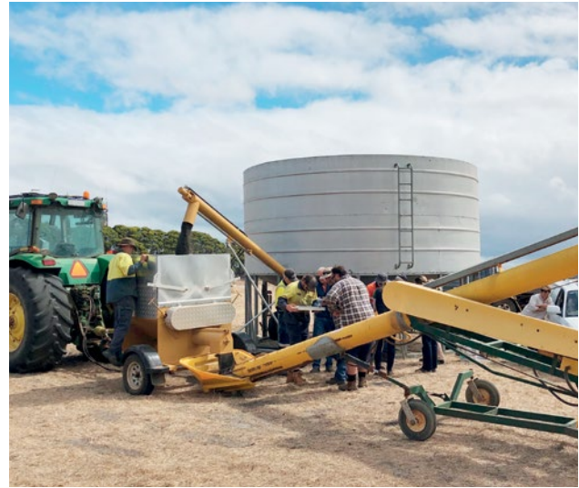
Figure 4: The SCF grain cleaning snail roller demonstration: cleaning snails out of barley. Further testing is required to provide growers with clear advice on the capacity of these rollers to remove small conical snails from grain.
