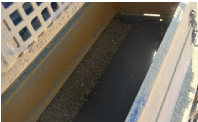
▲ Photo 2. The barley flowing between the rollers during sampling. The roller temperature may need to be monitored to make sure it does not exceed 65 °C. Using a gap of 0.8mm the roller temperature remained between 48-50 °C.
