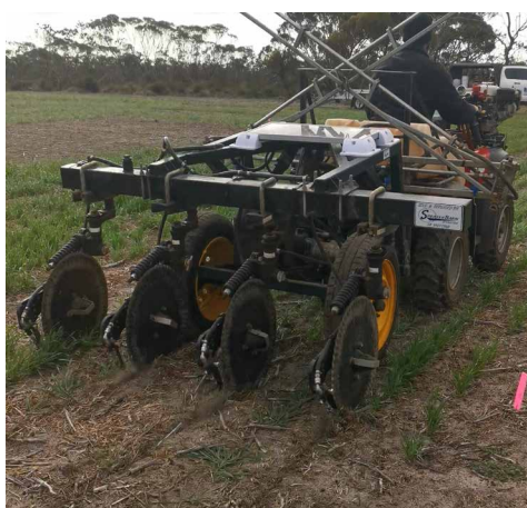
Figure 4: CSBP's trial mid-row banding machine
