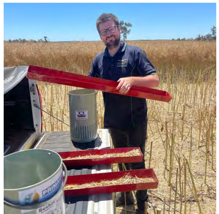
Figure 4. Placing losses through the Bushell Plus system
