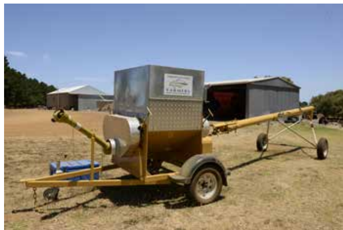
Snail-crushing grain rollers are used to remove snails from grain in parts of SA.
