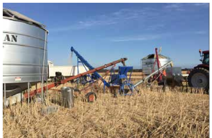
Grain cleaning set-up during harvest: grain goes from storage silo into grain cleaner, then through the snail roller and finally into a clean silo or straight onto a truck.
