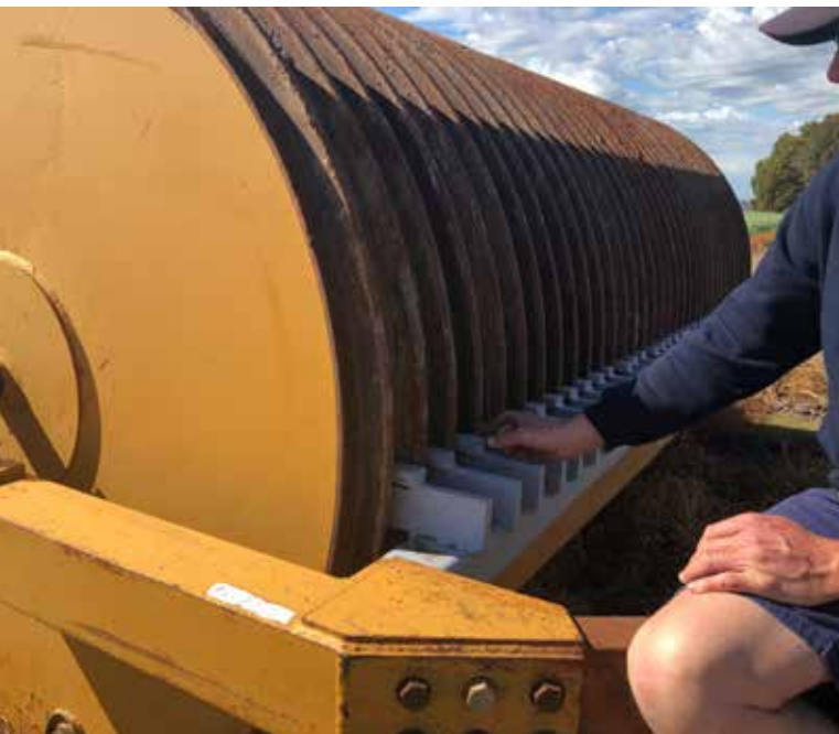
Ripple stone roller with modified part to dislodge dirt.
