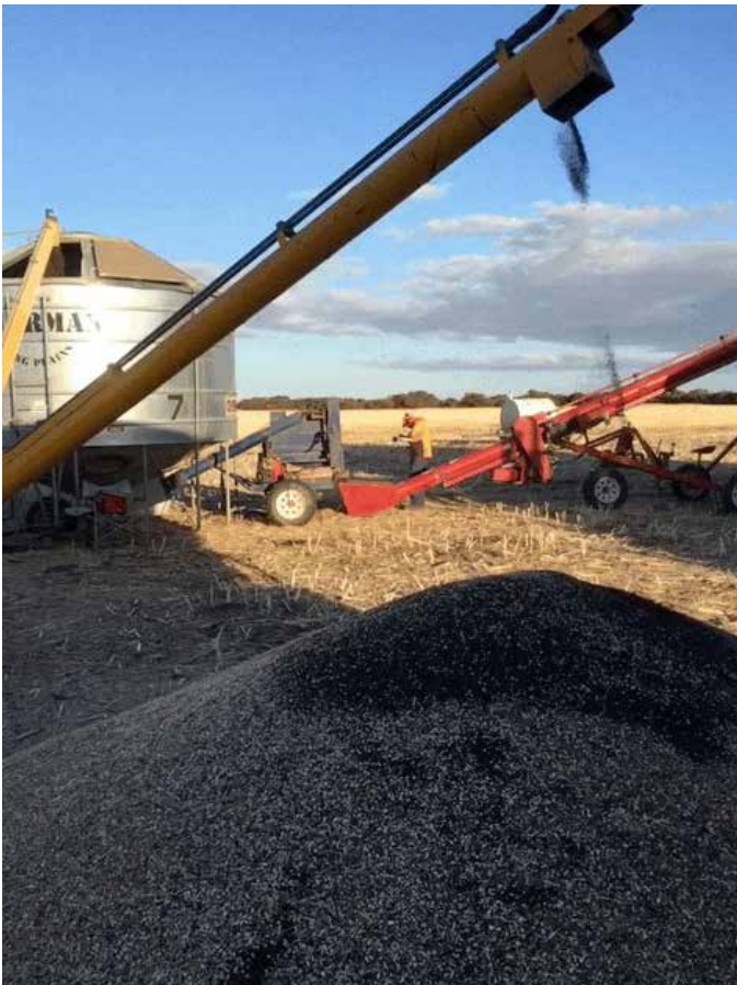
Snails cleaned out of grain in foreground and snail roller operating in background.
