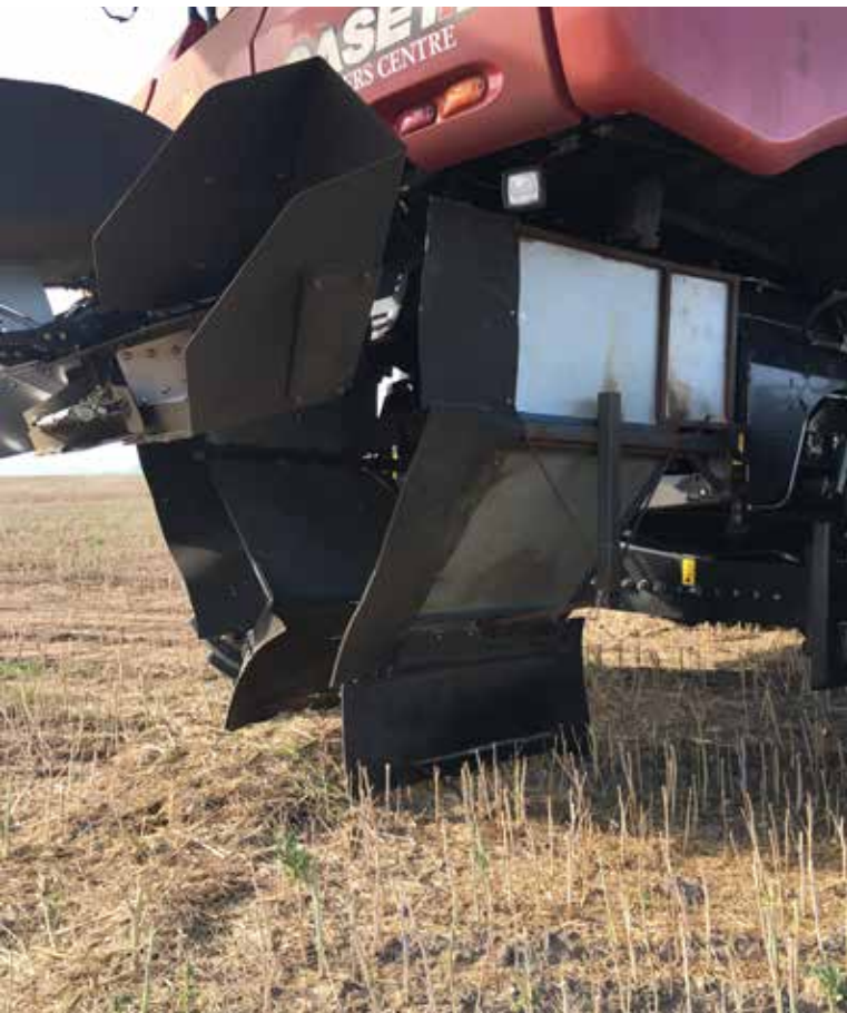
Chutes fitted to header to create narrow windrows in canola stubbles.
