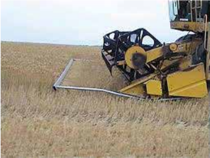
A dislodger bar fitted to the front of a header.
